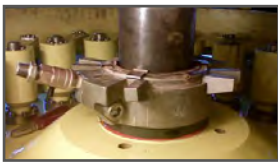
SpiralTrac Adaptor installed with a Chesterton 442HP Split Seal in a Hydro Turbine
