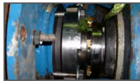
SpiralTrac Adaptor installed with a Chesterton S10 Seal in a Sulzer Scanpump®
