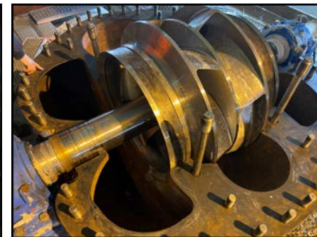
Originally packed equipment, excessive leakage issues and frequent sleeve replacements
