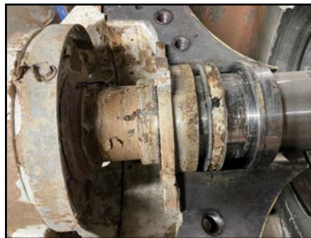
Originally packed equipment, excessive leakage issues and frequent sleeve replacements
