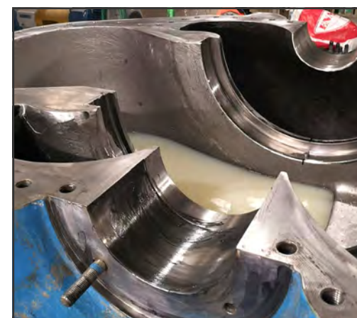
Pump disassembled, L-shaped bushing removed
