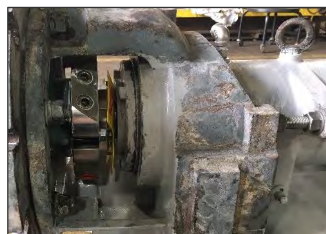
Chesterton solution installed in Furukawa SP2H-50 slurry pump
