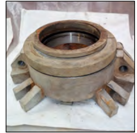
442 Split Seal and SpiralTrac Adaptor after 9 years of service
