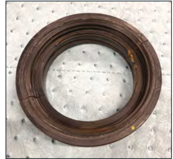
Worn SpiralTrac Adaptor after over 13 years in operation
