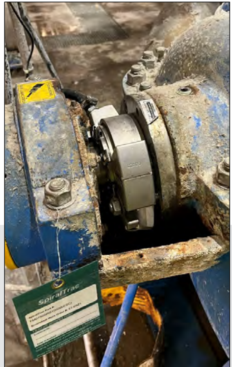
Chesterton solution installed, EnviroSeal green tag attached to rotating equipment
