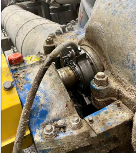
Chesterton solution installed, EnviroSeal green tag attached to rotating equipment
