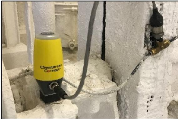
Chesterton Connect attached to slurry pump.
