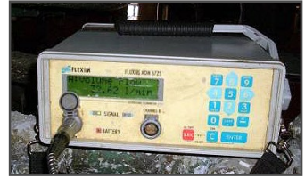
Flow monitor reading 32.62 l/min flush water usage
