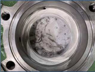
SpiralTrac pressed in at the bottom of seal cavity during installation
