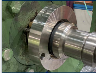
Chesterton 170 Seal being installed to pump housing
