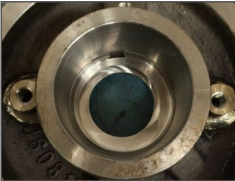
SpiralTrac installed at the bottom of the seal cavity
