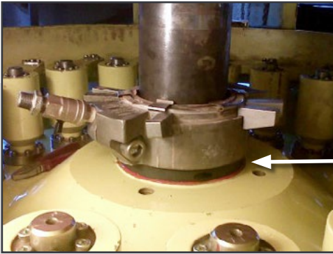
Chesterton 442HP seal installed on vertical turbine with the help of SpiralTrac Adaptor
