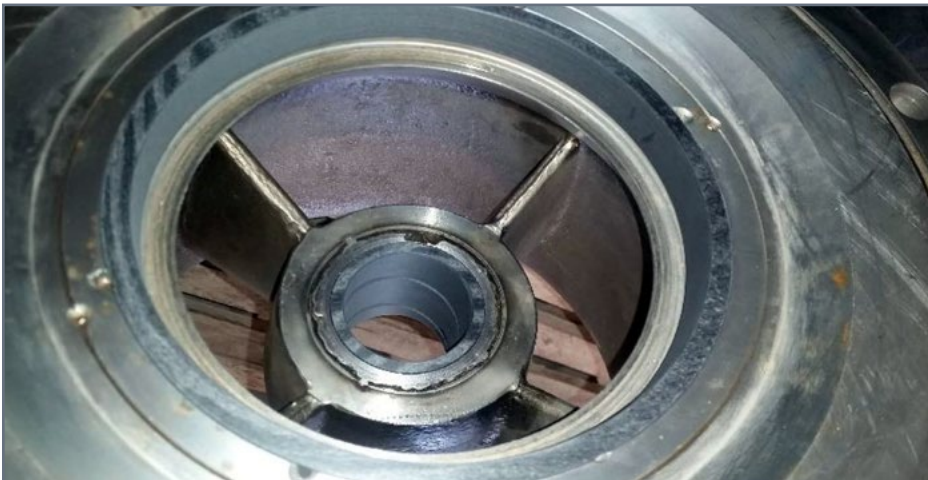
SpiralTrac press fit installation shown from the impeller side
