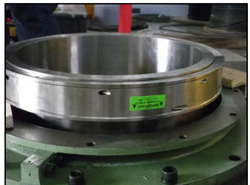
Split Wear Sleeve and Tri-split Stuffing Box assembly with SpiralTrac™
