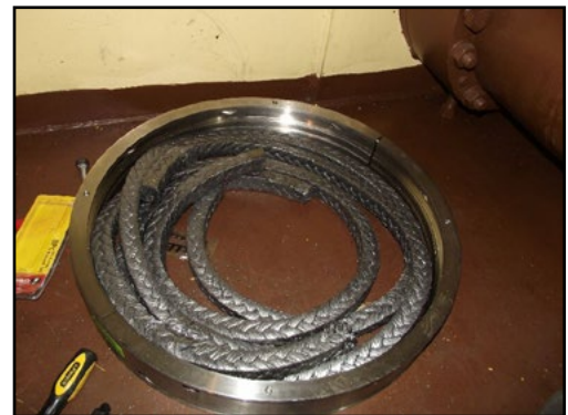
Chesterton SuperSet™: SpiralTrac™ Version P Split Metal Device with Chesterton 1400™ Graphite Packing
